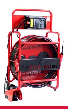
The Super Midi Miller is designed for cleaning, descaling, root removal, and cutting/reinstatements in DN70-150 (3-6") pipes. It has a range of 20m (65') that can be increased by an additional 10m (33') with a shaft extension. It can also be paired with the Picote Maxi Coating Pump to coat pipes DN70-200 (3-8").
