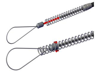
• To remove the tool, loosen the set screws and follow the previous steps in reverse order.
