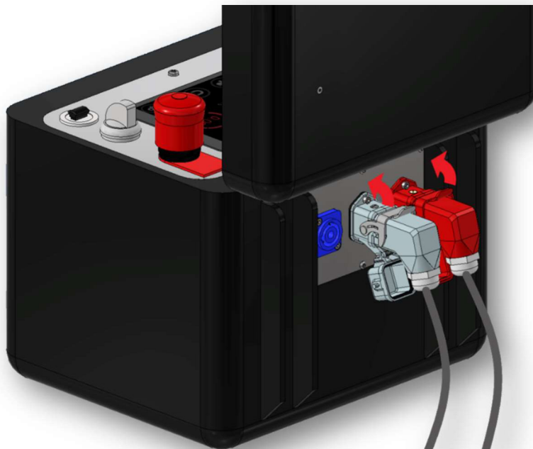
Figure 28 Push up the safety bar
