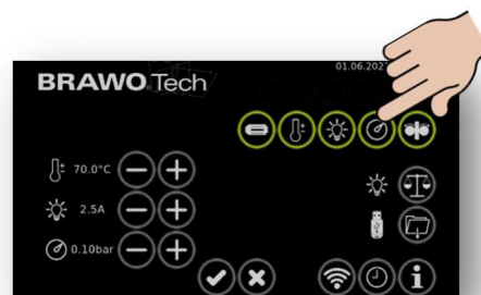
Figure 114 Switch on working pressure monitoring
