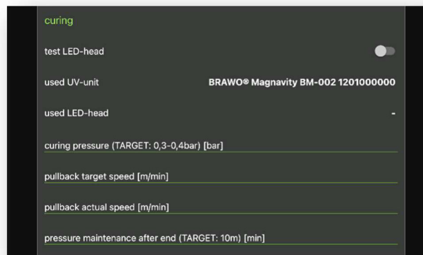
Figure 91 Log management “Curing”
