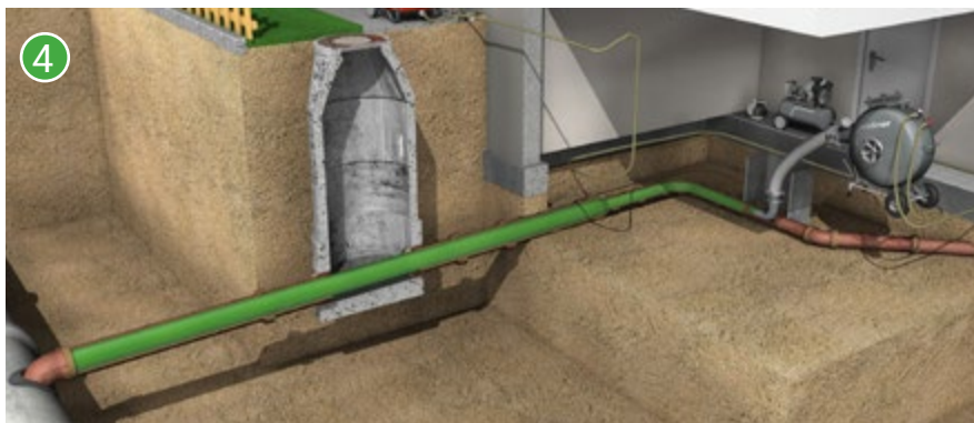
Result after curing: a new pipe in the old pipe
